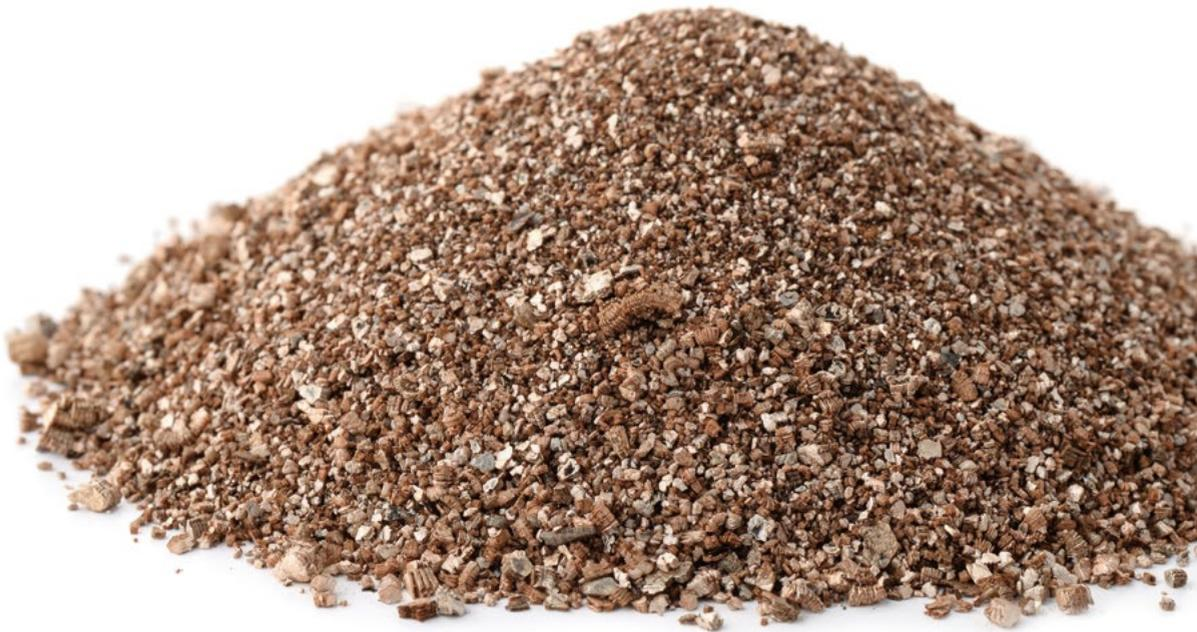
Figura 20 - Vermiculita Expandida a granel
